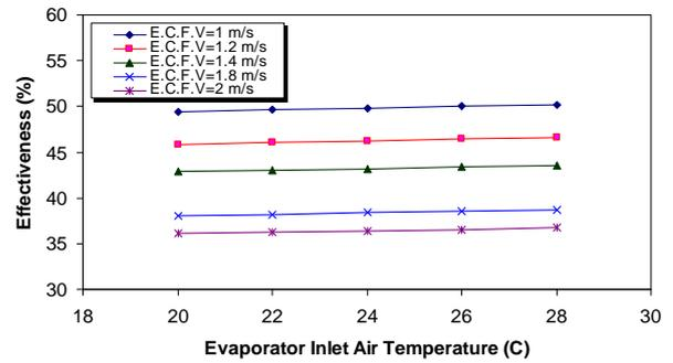
Figure 3. Effectiveness vs. evaporator inlet air temperature for typical two rows
