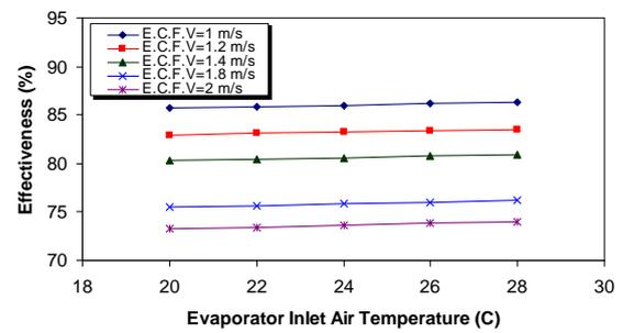
Figure 4. Effectiveness vs. evaporator inlet air temperature for typical four rows
