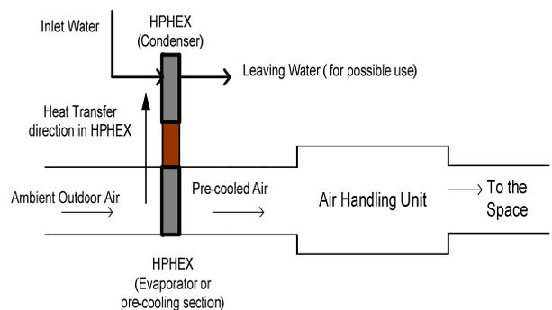
Figure 9. Schematic diagram of the pre-cooling process in an air-conditioning system (top view)
