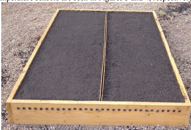
Figure 2. The asphalt solar collector under consideration
