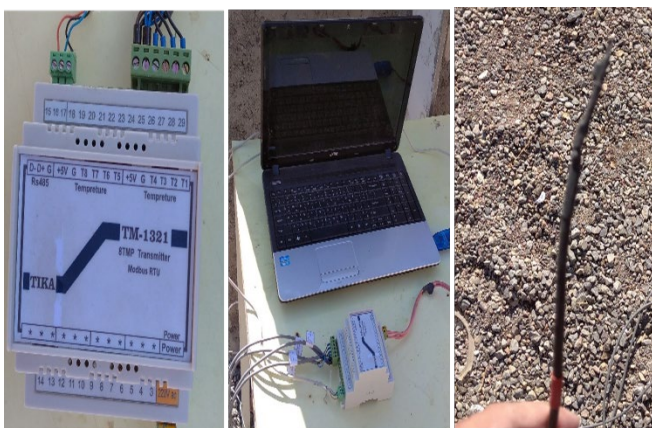
Figure 4. Temperature sensor and transmitter type TM-1321
