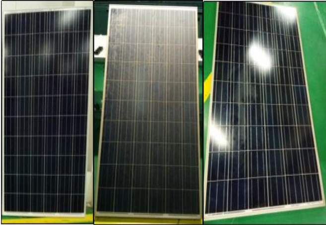
Figure 1. Used panels from left to right : (a) Reference panel, (b) degraded panel with dust and (c) degraded panel without dust.
