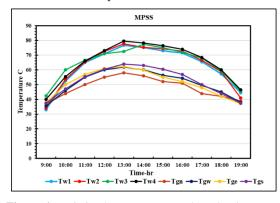
Figure 6. Variation between water and condensing cover temperatures in MPSS.
