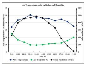
Figure 4. Variation between outside condition with time.
