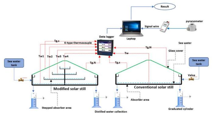
Figure 1. Schematic diagram of the proposed system.
