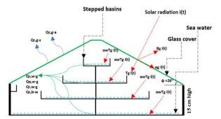
Figure 3. Schematic of the heat flow through the parts of MPSS.
