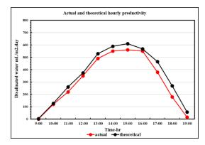
Figure 9. Theoretical/experimental results of distillate output.
