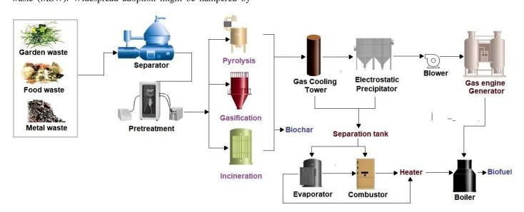
Figure 6. Thermal conversion of organic fraction of municipal solid waste
