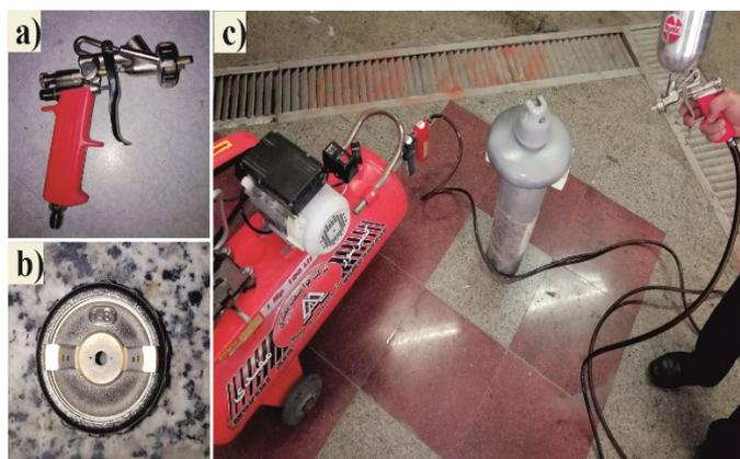
**Figure 3.** a) Gun used for spraying, b) Nozzles with a diameter of 1.8 mm, and c) Equipment needed for insulator coating operations
