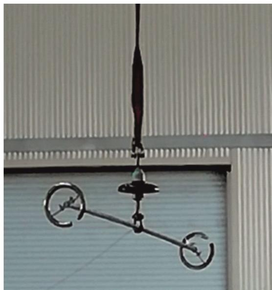
**Figure 5.** Insulator mounted for electrical testing
