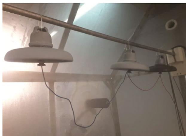
**Figure 9.** Samples in the salt fog chamber
