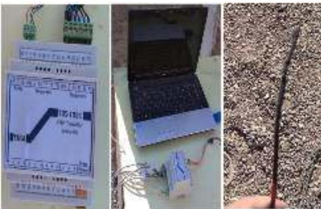
Figure 4. Temperature sensor and transmitter type TM-1321
