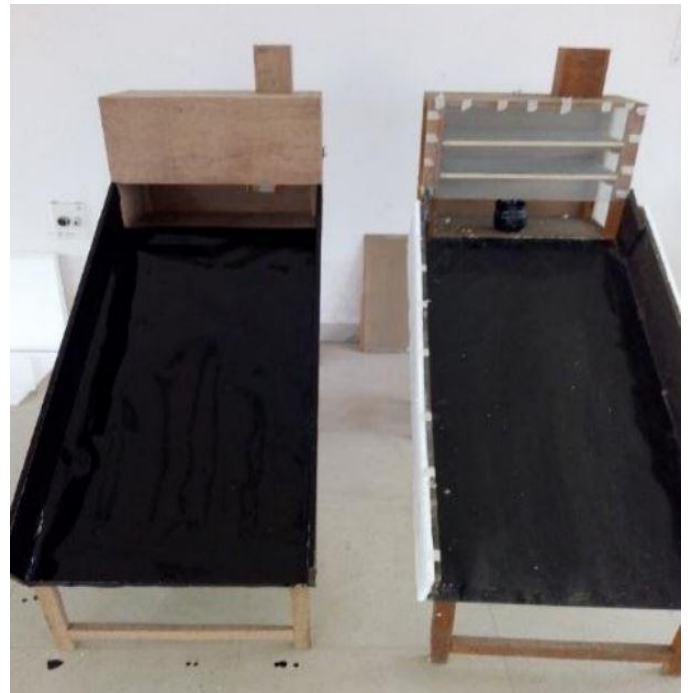
Figure 13. Indirect and mixed mode solar dryers with phase change material (Singh & Mall, 2018)
