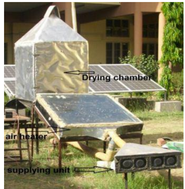
Figure 3. Photographic view of drying of fenugreek in forced convection indirect solar dryer (Shrivastava & Kumar, 2016)
