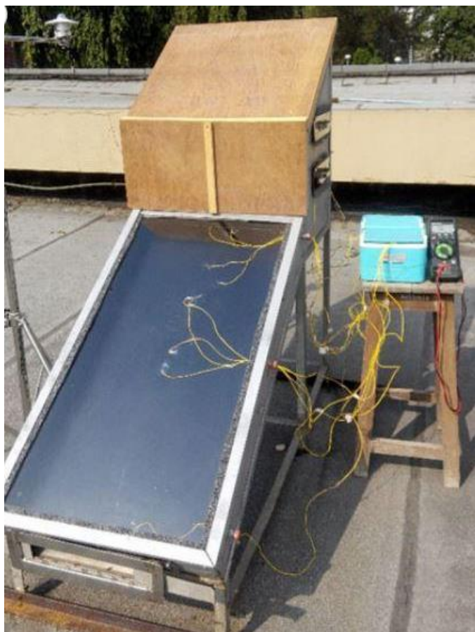
Figure 4. Indirect solar dryer for drying carrot slices (Mahapatra & Tripathy, 2018)
