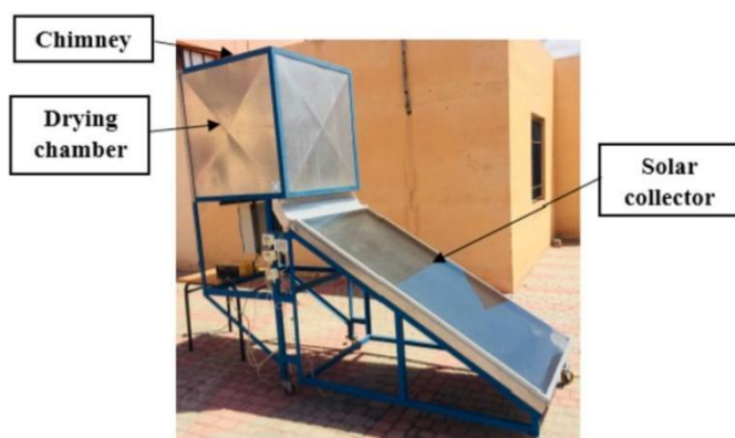
Figure 2. The experimental rig (Zoukit et al., 2019)
