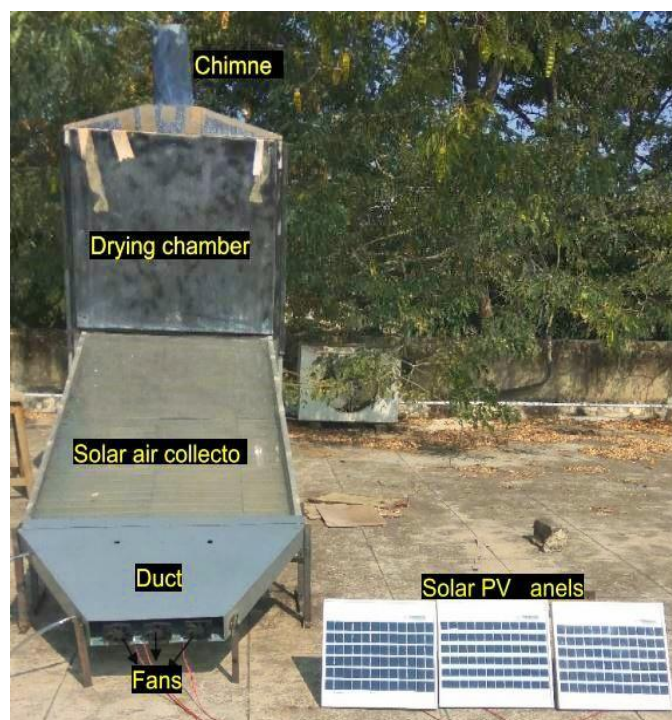
Figure 5. Indirect-type solar dryer with V corrugated absorber surface coupled with the trapezoidal duct (Goud et al., 2019)
