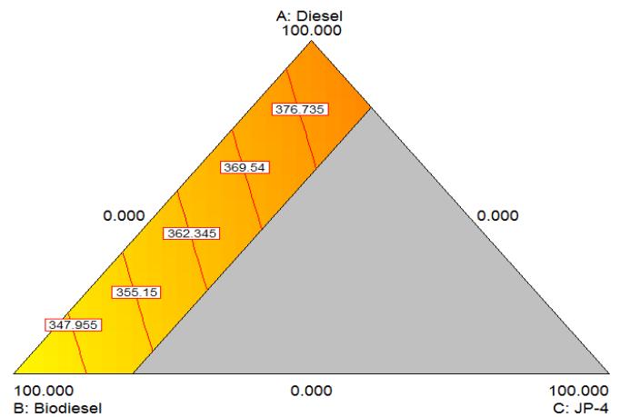
Figure 12. Brake torque variations at a speed of 2250 rpm and full load.
