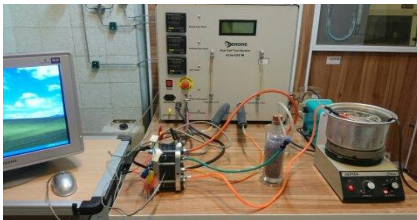
Figure 2. Photograph of the DMFC stack test station.
