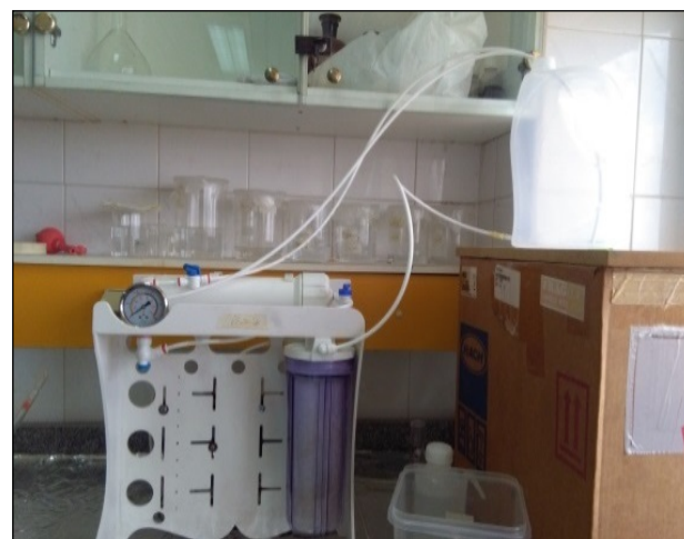
Figure 2b. Actual photo of the RO system pilot for the desalination and TOC removal test.
