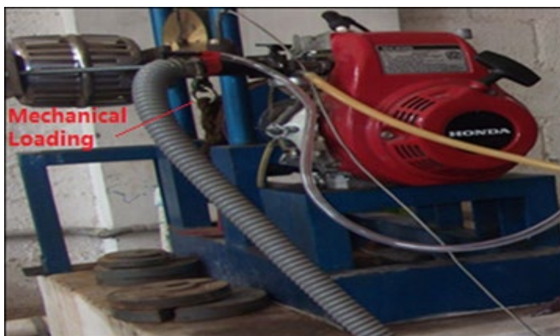
(c) Experimental engine setup with loading setup
