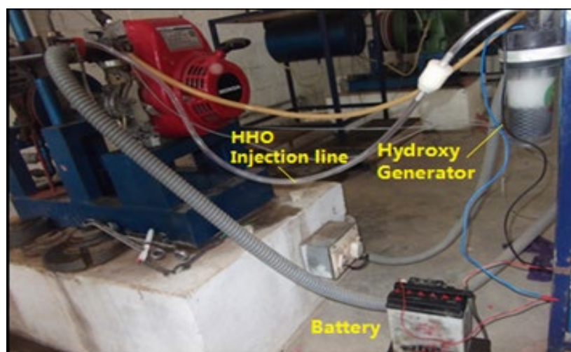
(b) Experimental engine setup with Hydroxy gas
