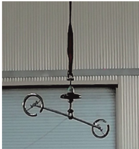
Figure 5. Insulator mounted for electrical testing
