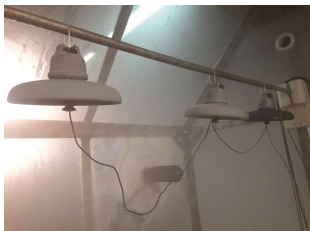
Figure 9. Samples in the salt fog chamber
