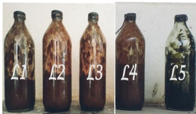
Figure 2. The experimental setup containing a mixture of cow dung and water hyacinth food waste
