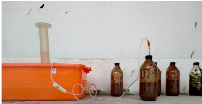
Figure 3. The laboratory setup was prepared with different substrates-L1 (CD), L2 (CD: WH), L3 (CD: FW), L4 (CD:WH: FW), L5 (WH)
