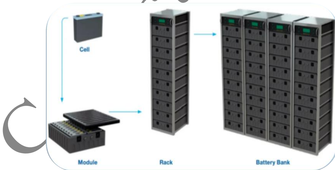
Figure 4. Modularity of LFP batteries [12]
