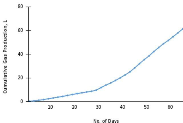
**Figure 5.** Cumulative Biogas Production in ambient temperature conditions
