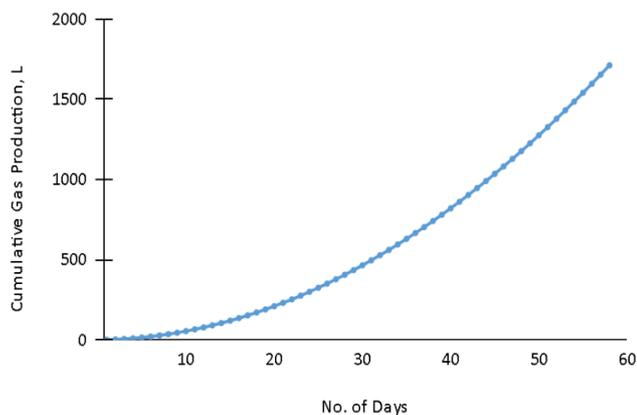
**Figure 3.** Cumulative biogas production at controlled temperature
