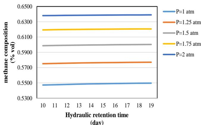
**Figure 2.** Effect of retention time on composition of biogas at different digestion pressures
