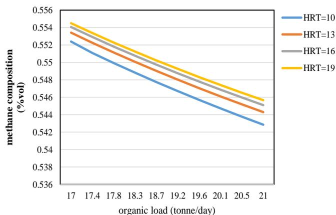
**Figure 7.** Effect of OLR on composition of biogas at different retention times
