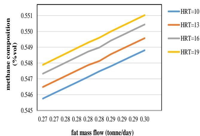
Figure 4. Effect of lipid on biogas composition of at different retention times
