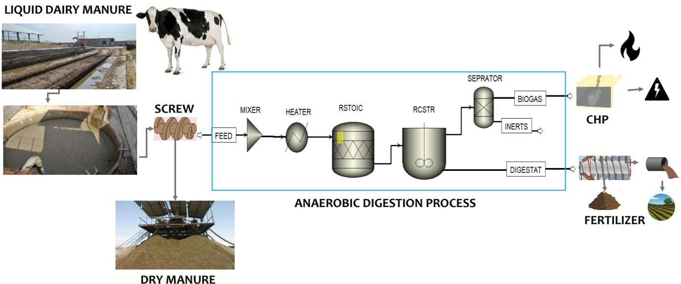
Figure 1. Schematic of anaerobic digestion process from raw material to end products
