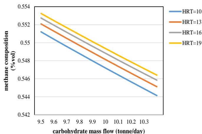
Figure 3. Effect of carbohydrate rate on the composition of biogas at different retention times
