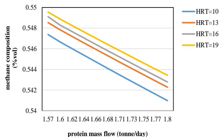
Figure 5. Methane composition as a function of mass protein rate at different retention times
