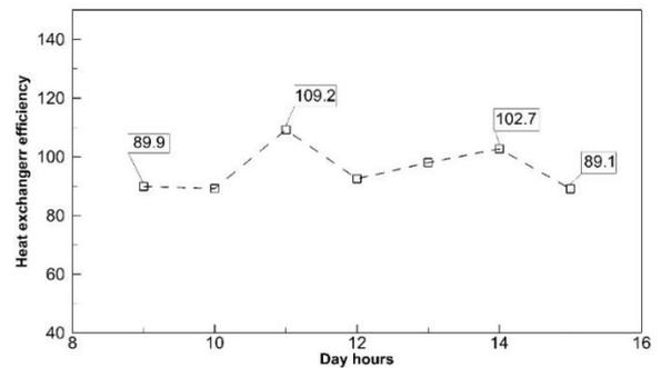
**Figure 14.** Heat exchanger efficiency diagram when connected to PVT solar collectors.
