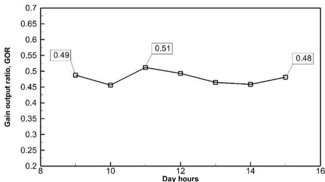
**Figure 12.** The graph of the output ratio obtained when connected to PVT solar collectors.
