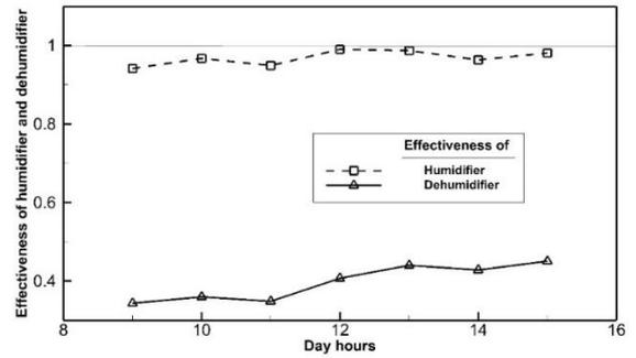
**Figure 13.** Effectiveness diagram of humidifier and dehumidifier towers when connected to PVT solar collectors.
