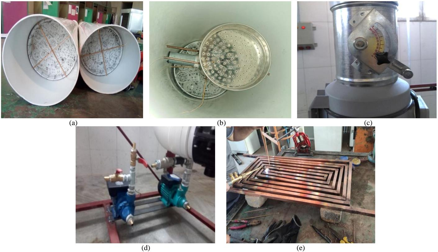
**Figure 2.** a) Interior view of humidifier and dehumidifier towers, b) Nozzle installation location in towers, c) Inter-channel and damp channel fan installed on the device, d) Water pumps for water circulation in the cycle, e) Construction of PVT collectors
