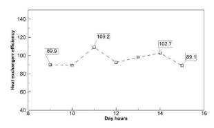
**Figure 14.** Heat exchanger efficiency diagram when connected to PVT solar collectors.
