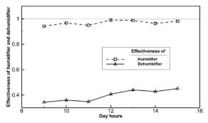
Figure 13. Effectiveness diagram of humidifier and dehumidifier towers when connected to PVT solar collectors.
