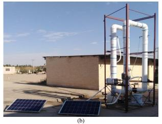
Figure 3. Desalination system (a) without and (b) with connection to PVT collectors
