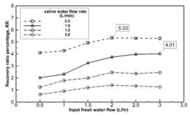
**Figure 6.** Recovery ratio at different discharges of saline water and fresh water, damper angle 30° without connection to PVT solar
