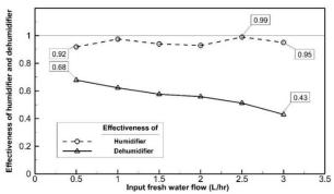
**Figure 8.** Diagram of the effectiveness of humidifier and dehumidifier towers in different saline and fresh water discharges without connection to PVT solar collectors
