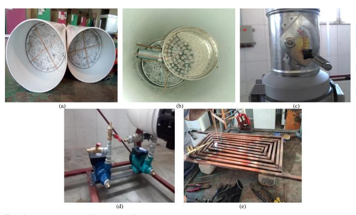
**Figure 2.** a) Interior view of humidifier and dehumidifier towers, b) Nozzle installation location in towers. C) Inter-channel and damp channel fan installed on the device, d) Water pumps for water circulation in the cycle, e) Construction of PVT collectors
