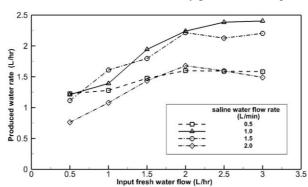
**Figure 5.** Diagram of water production rate at different discharges of saline water and fresh water, 30° angle of channel damper in case of no connection to PVT solar collectors
