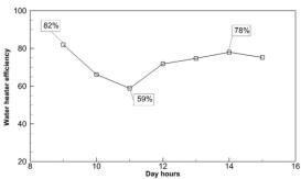
**Figure 15.** Efficiency diagram of water heater connected to PVT solar collectors
