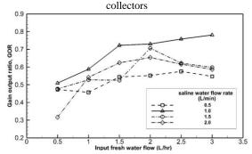
**Figure 7.** Diagram of the gain output ratio in different streams of saline and fresh water in the state without connection to PVT solar collectors
