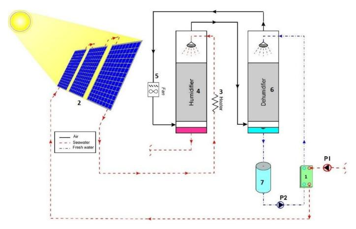
Figure 1. . Schematic view of a water-desalination system with closed air cycle - open water with water preheating and photovoltaic panel
