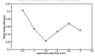
**Figure 9.** Water heater efficiency diagram without connection to PVT solar collectors
