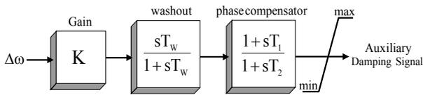
Figure 5. Auxiliary SSRD controller structure.
