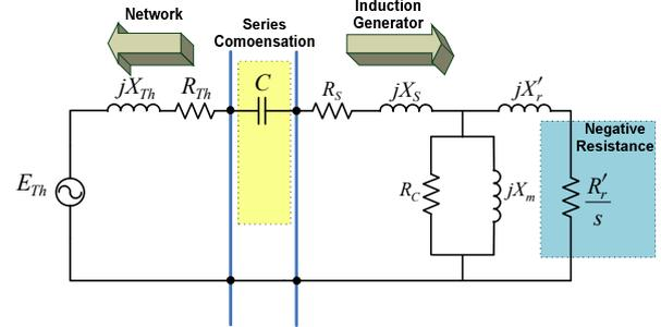
**Figure 1.** Equivalent circuit of a wind driven induction generator integrated to the main grid.
