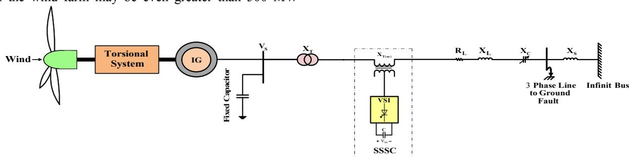
Figure 2. Wind farm comprises SSSC connected to a series compensated power system.
