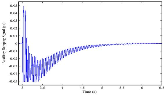
**Figure 7.** Auxiliary signal added to the voltage reference value.
