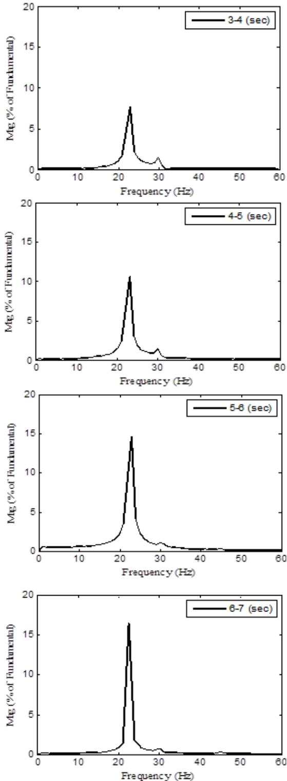
**Figure 3.** FFT analysis on generator rotor speed (non-FACTS power system).
