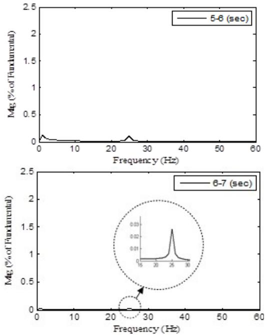
**Figure 8.** FFT analysis on generator rotor speed (SSSC equipped with SSRD controller).
