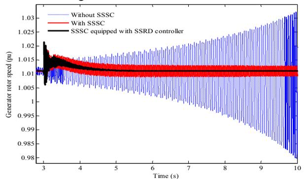
Figure 6. Mitigating IG effect, rotor speed behavior.
