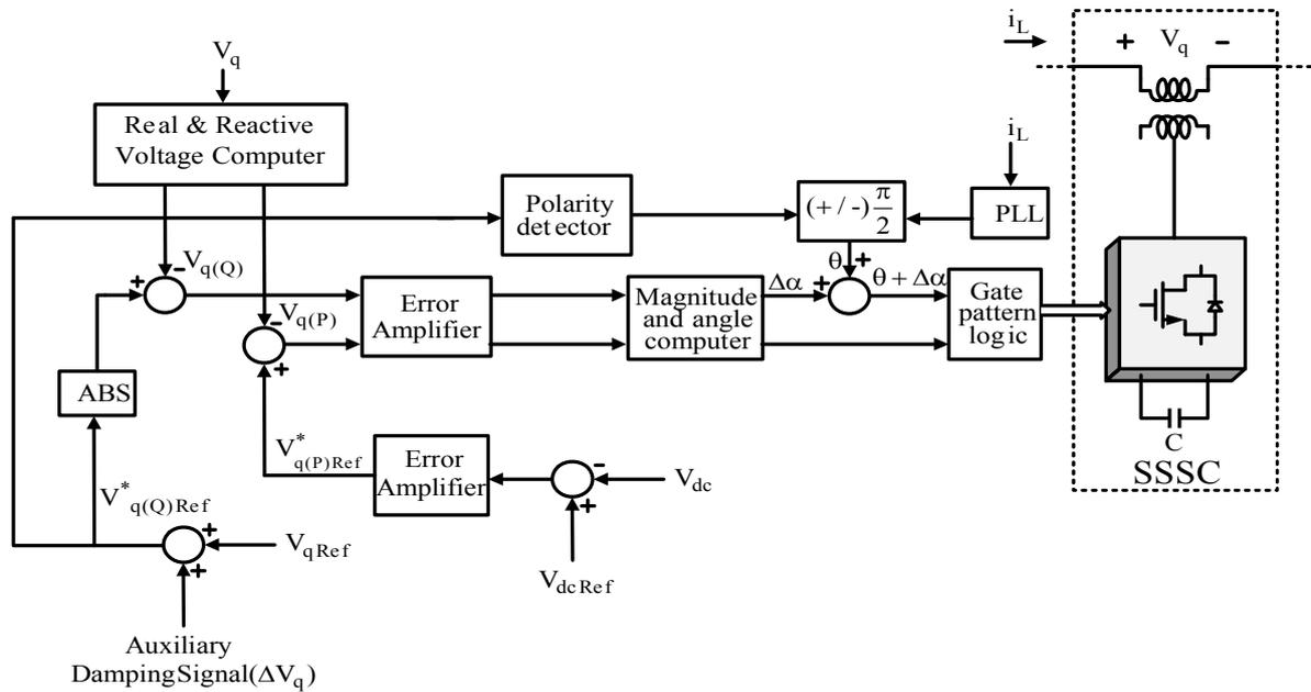
Figure 4. The SSSC main control system.
