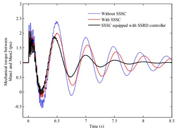
**Figure 9.** TIs mitigation (a) generator rotor speed (b) mechanical torque in multimass system.
