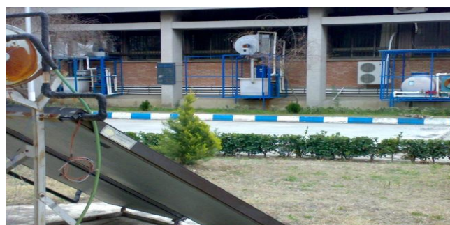
Figure 21. Flat plate solar collectors used for heating and regeneration of dilute liquid desiccant
