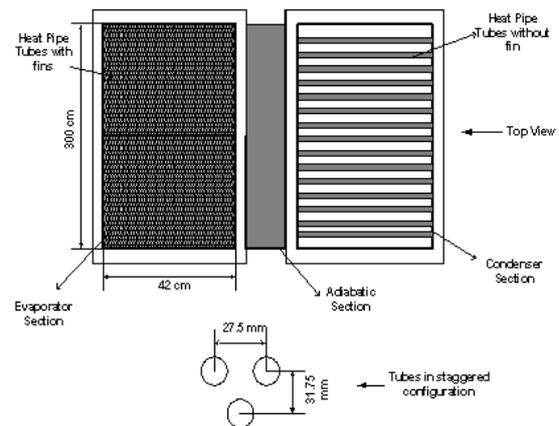
Figure 2. Schematic diagram of the air-to-water HPHEXs
