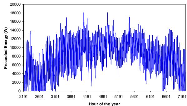
Figure 14. Hourly air pre-cooling by the six rows air-to-water HPHEX at 24 °C condenser. inlet temperature and 1 m / s coil face velocity for Bandar Abbas
