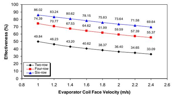
Figure 5. Effectiveness vs. evaporator coil face velocity for typical six rows
