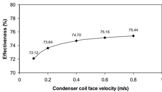
Figure 7. Effectiveness vs. condenser coil face velocity for typical six rows
