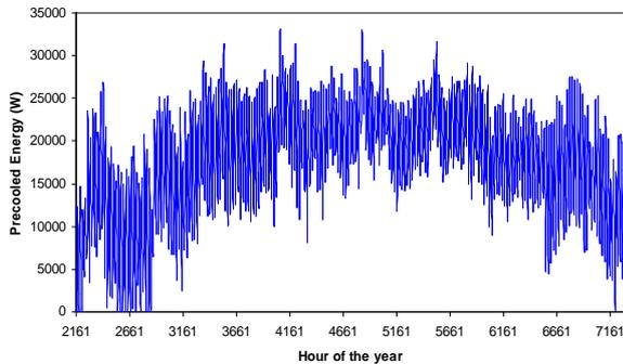
Figure 13. Hourly air pre-cooling by the six rows air-to-water HPHEX at 20 °C condenser. inlet temperature and 1.5 m / s coil face velocity for Bandar Abbas
