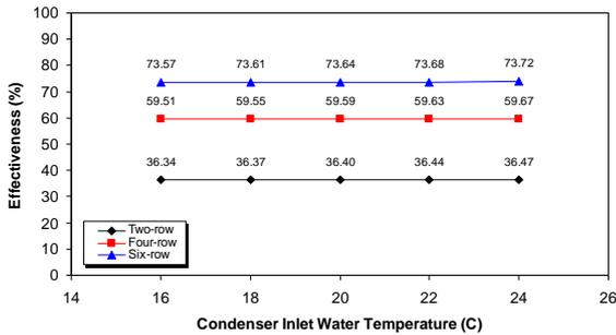
Figure 6. Effectiveness vs. condenser inlet water temperature
