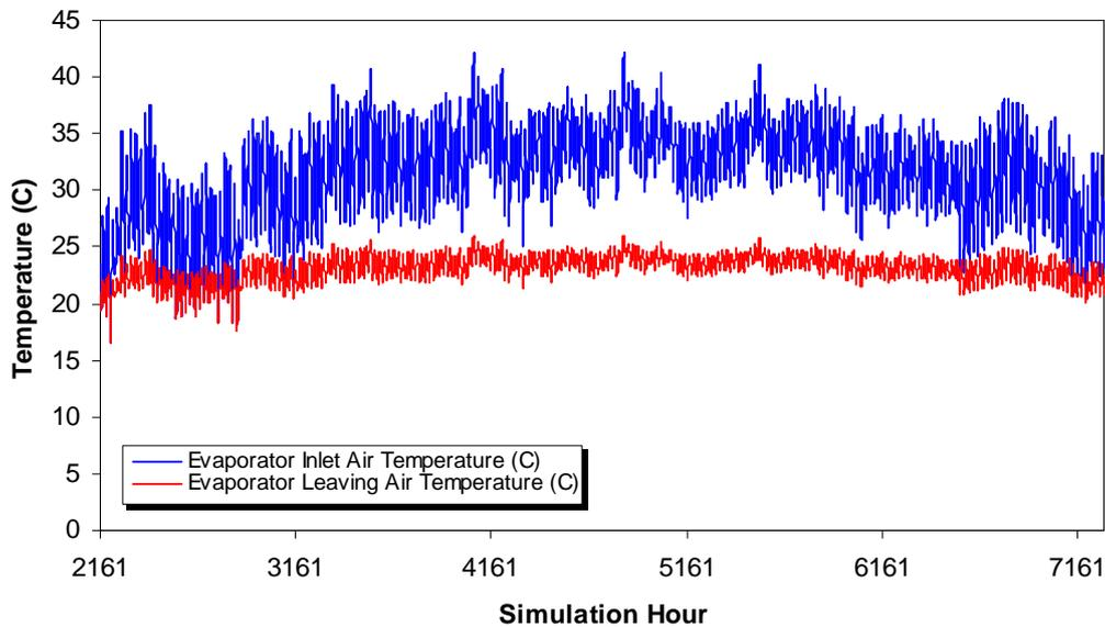
Figure 12. Hourly temperature reduction by the evaporator section of the six rows air-to-water
