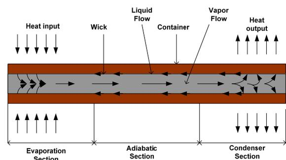
**Figure 1.** A schematic diagram of a heat pipe structure
