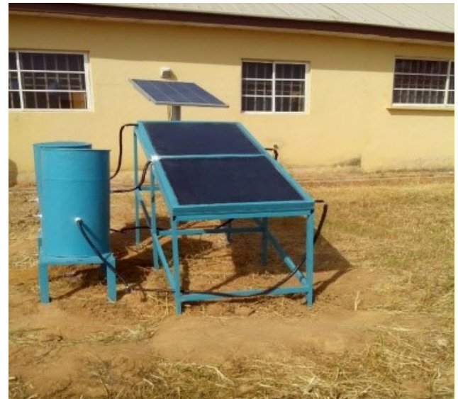
Figure 6. The developed and installed solar heating experimental setup
