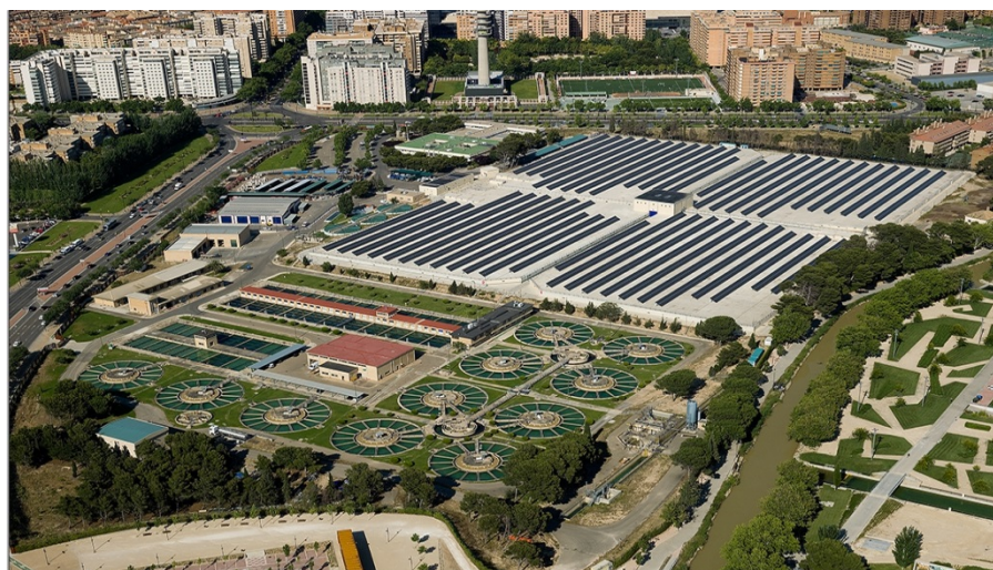
Figure 3. A water storage tank covered by solar photovoltaic panels [31].
