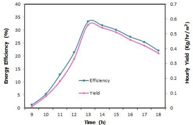
Figure 5. Effect of hourly yield and energy efficiency with time
