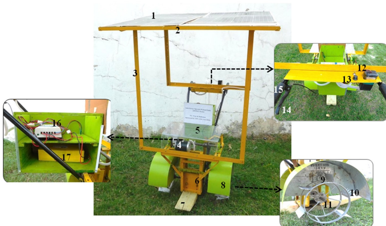
1. Solar panels; 2. Panel holding frame; 3. Stand for frame; 4. DC motor; 5. Transparent protection; 6. Main frame; 7. Float; 8. Mud guard; 9. Weeding wheel; 10. Weeding elements; 11. Rotating shaft; 12. ON/OFF switch; 13. Speed regulator; 14. Clutch lever; 15. Handle; 16. MPPT; 17. Battery
