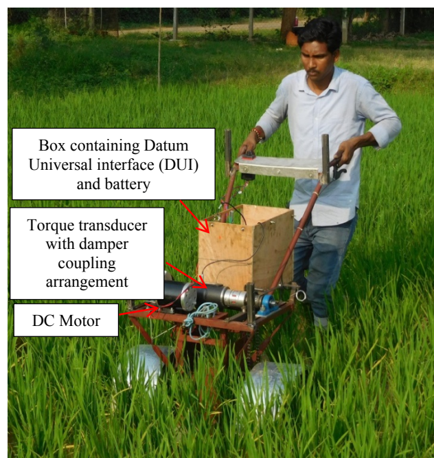
Figure 2. The developed wetland paddy weeder
