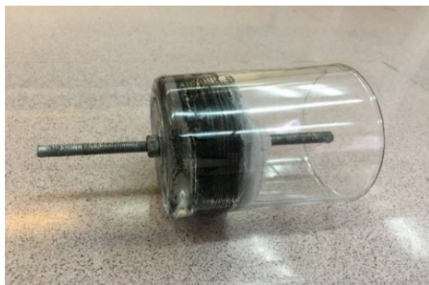
Figure 2. Picture of the cylindrical glass container for electrical resistance testing
