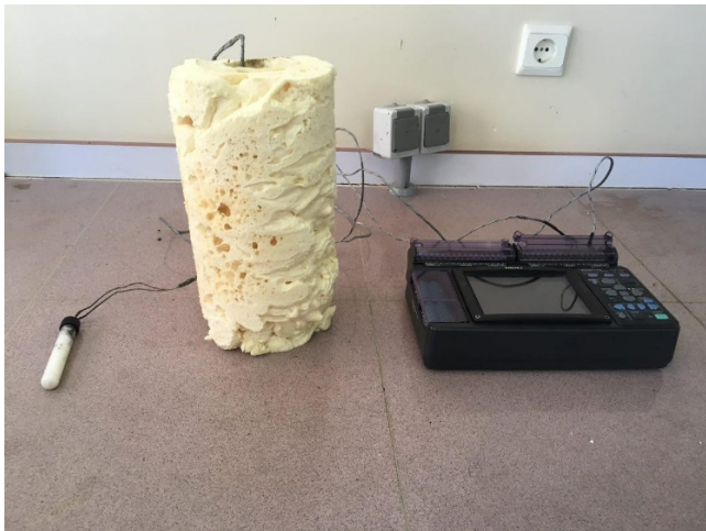
Figure 5. Picture of the insulated flask and measuring heat release rate test setup
