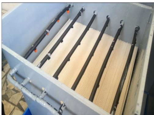
Figure 5. A photograph of the dehumidification tower used in the enthalpy exchanger.
