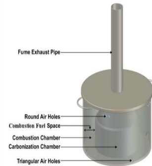
Fig.1: A 3D representation of top-lit updraft gasifier (TLUG)
