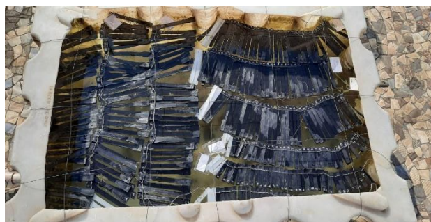
Figure 02 The weathering of the sample out of water (left figure) and the weathering of the sample in water (right figure).
