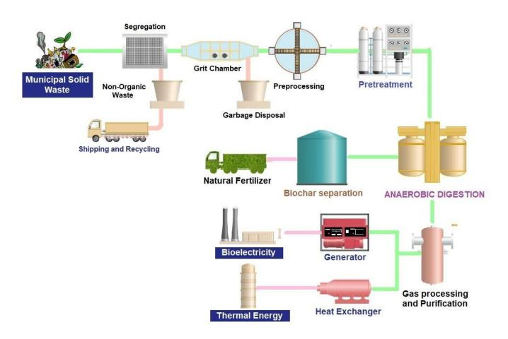
Figure 7. Steps involved in anaerobic digestion based treatment of municipal solid waste
