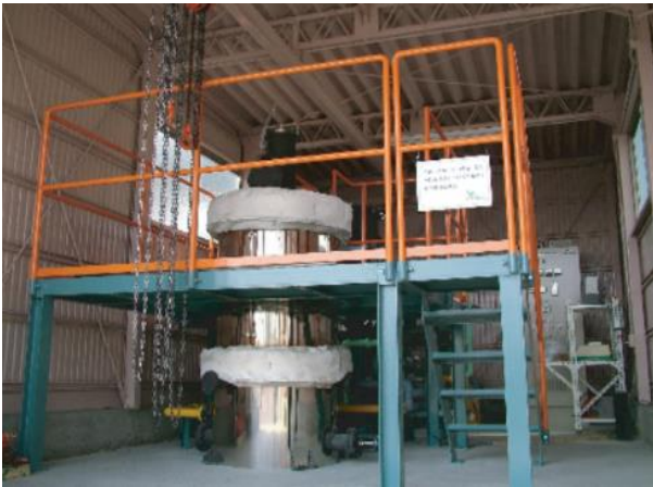
Figure 5. Biomass gasification system
